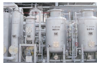
Equipment for recovery of carbon disulfide (Marugame Plant)
