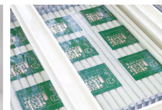
PWBs treated with Glicoat-SMD
