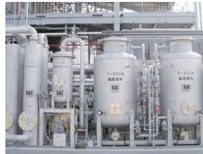
Equipment for recovery of carbon disulfide (Marugame Plant)
