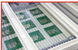
■ Printed wiring boards going through Gliccoat-SMD treatment tank
